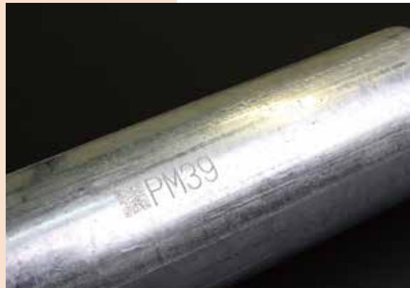
Mark 2D code on pipe.
